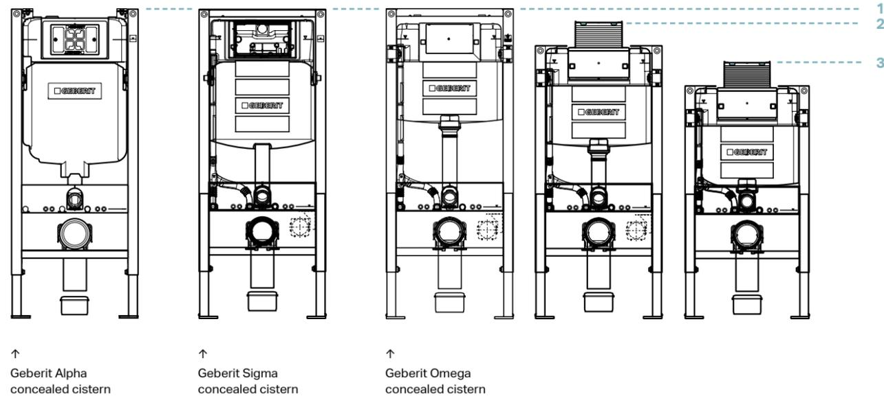
1 Construction height 112 cm. 2 Construction height 98 cm. 3 Construction height 82 cm.
