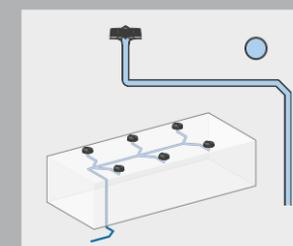
↑ Geberit Pluvia syphonic roof drainage
