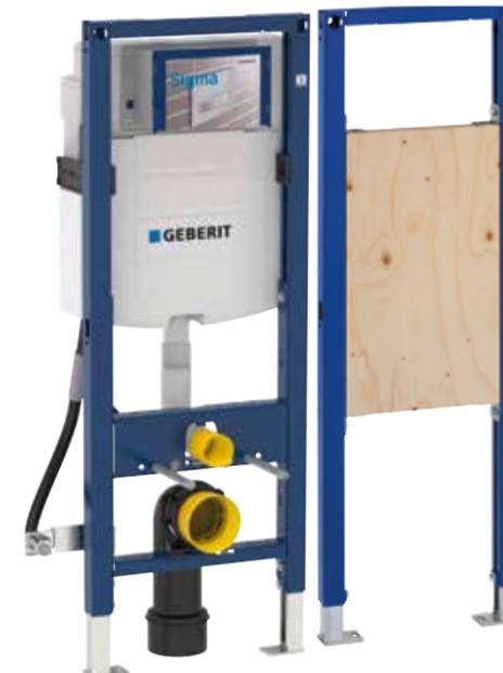
← GEBERIT DUOFIX ELEMENT FOR WALL-HUNG WC C BARRIER-FREE For height-adjustable wall-hung WC with mounting plates for support handles.
